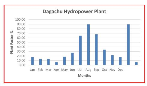
Graph: 2.2.4 Plant factor of Dagachhu Hydropower Plant
